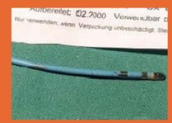
heart valve was locked between the electrodes. Image- Eucomed
