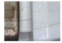
The white plastic tip of a linear cutter has become separated slightly, exhibiting a crack and blood and body fluid residues
